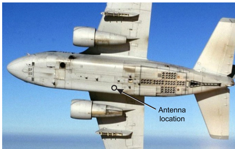
Figure 7.—Aircraft antenna placement.
