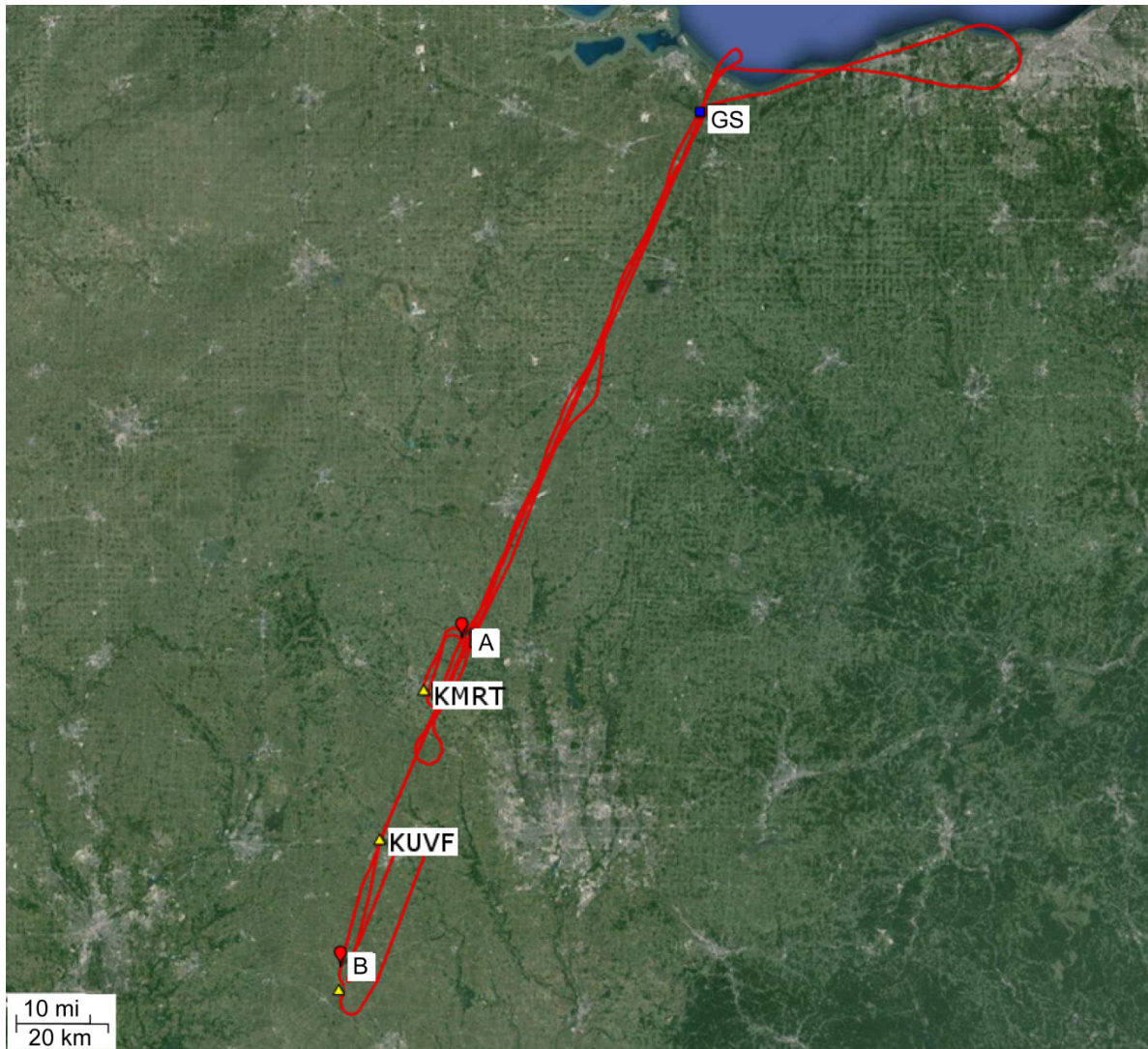
Figure 13.—Research flight track for Flight Test 2—May 23, 2013; GS, ground system; KMRT, Union County Airport; KUVF, Madison County Airport; B, region of signal loss. Map created at GPSVisualizer.com. Imaging ©2013 TerraMetrics.
