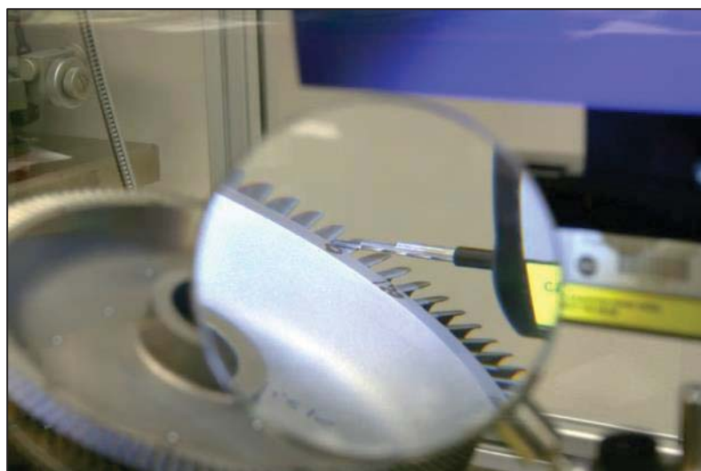
Stylus profiling of Blisk Blade (EM10-Tribology)
