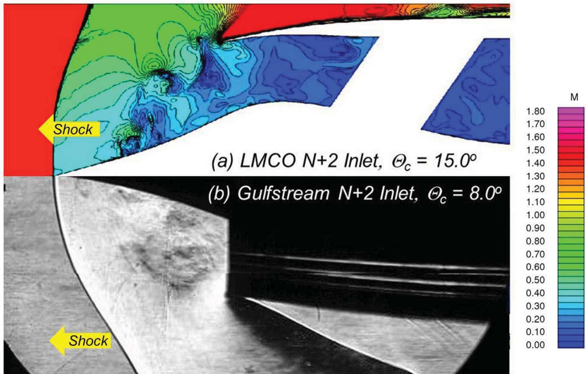
Figure (16): Comparison of CFD analysis and Schlieren photograph during buzz cycle, \Delta t = 3.0 \times 10^{-3} sec.
