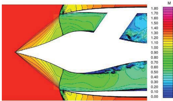
Figure (6): Typical DES analysis phase (1) inlet operations, streamwise Mach number contours.
