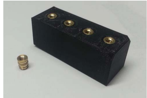
Figure 6. Heat Set Inserts. Four inserts installed in test block and one insert not installed.
