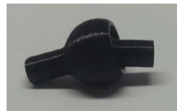
Figure 5. Section view of second joint concept and printed model. (Top) In red the single piece cup end and in blue, the ball end (Bottom) Completed print of ball joint
