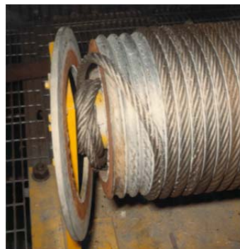
Figure 13. Separated end plate on Winch #6. 11 Note cable wrapped on shaft.
