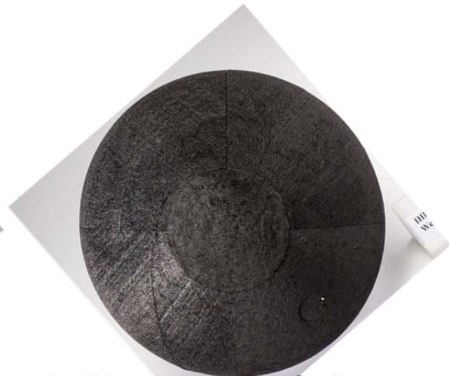
Flank heating ~400 W/cm 2 , 30 s Flank shear ~200 Pa Shoulder shear ~500 Pa
