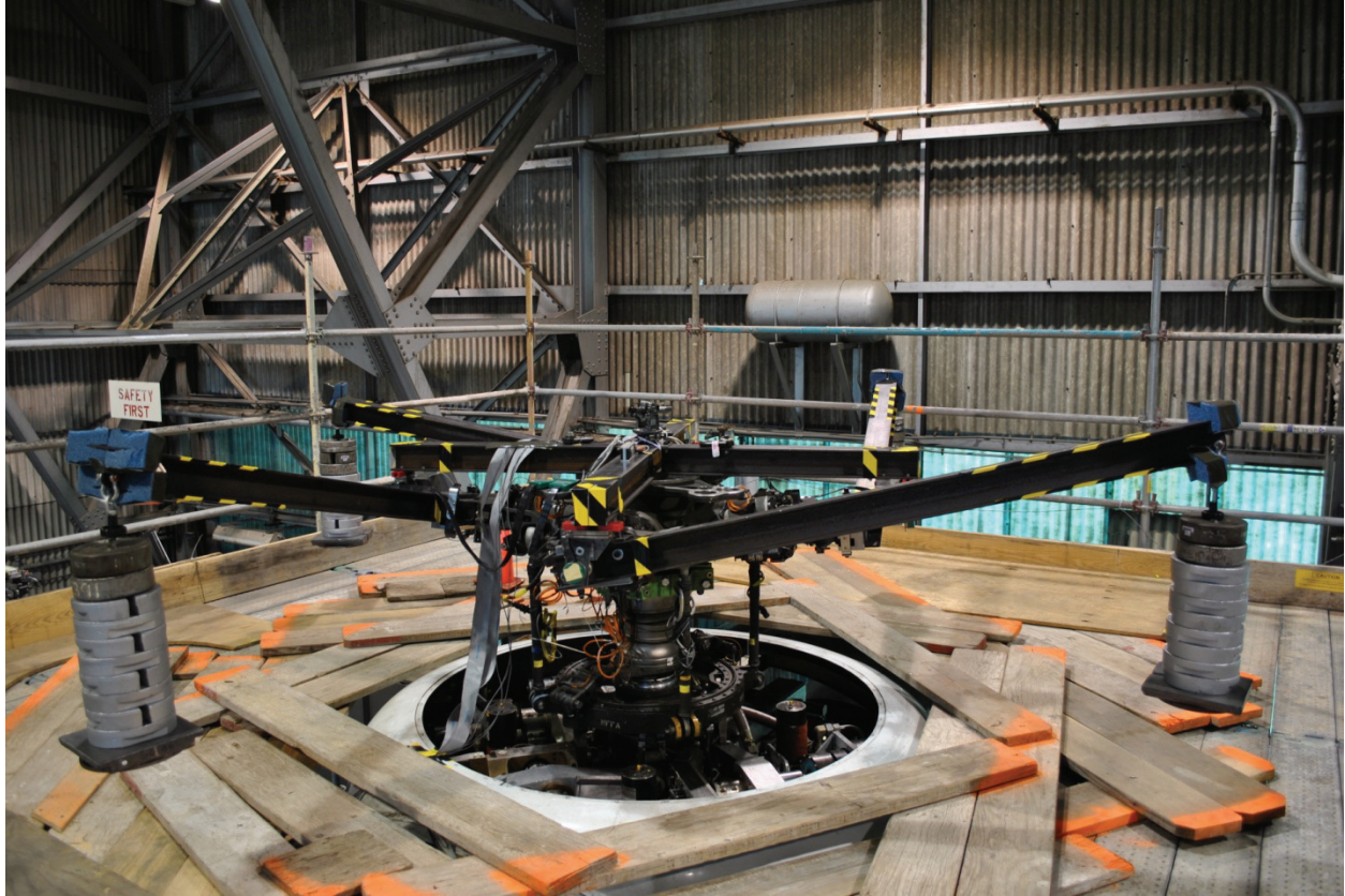
Figure 13. Maximum collective loading condition, 250 pounds hanging from all four moment arms.
