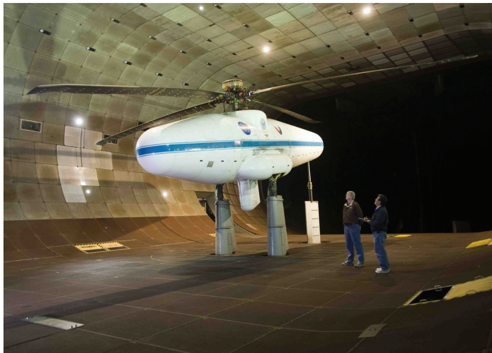
Figure 1. UH-60A Airloads rotor mounted on the LRTA inside the NFAC 40- by 80-Foot Wind Tunnel.
