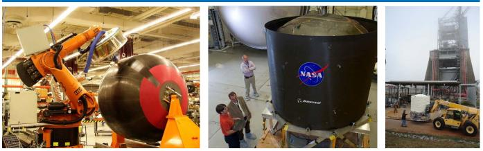
A robotic arm applies composite laminate (Cytec CYCOM<sup>®</sup> 5320-1 pre-preg) to the tank at Boeing's Development Center in Washington.
