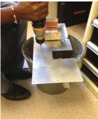
Figure 10. Plate drilling. Here we are drilling holes in the plate so we can mount the avionics.
