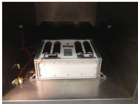
Figure 14. Thermal testing. This is EMIST inside of the thermal vacuum chamber.
