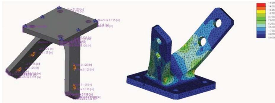
Figure 19. FEM (left) and FEA results (right) of the Angle Beams-to-Wide Flange Adapter. The Von Mises Stresses, ksi, fringe plot is scaled such that the color red denotes an area of the material violating the required factor of safety.
