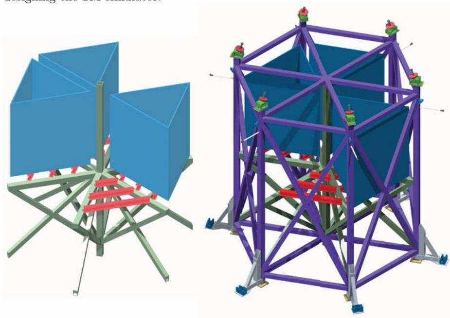
**Figure 6.** Creo renderings of the first simulator concept alone and installed inside the SM. Color Scheme: (Blue) Water Tanks (Red) Floor Support (Green) Structural Members, which connect inside the SM structure (Purple) SM Structure.
