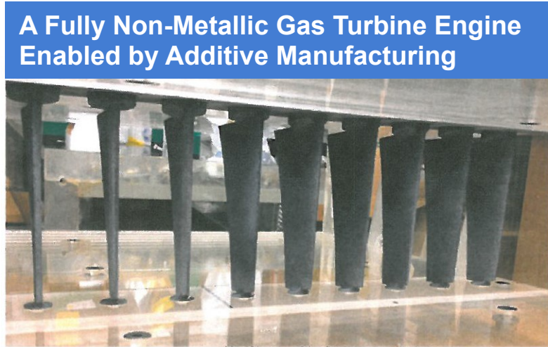
Polymer Vane Configuration in Cascade wind tunnel Rig
