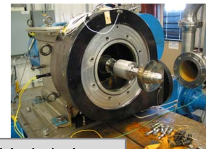
2-blade inducer with on-rotor dynamic force measurement system
