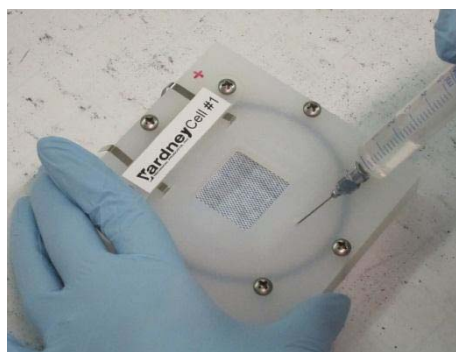
Figure 4: Activation of a Yardney cell with electrolyte
