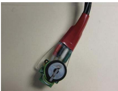
Figure 1: Representative coin cell by Ionova. Shown in holder and connected to current and sense leads.
