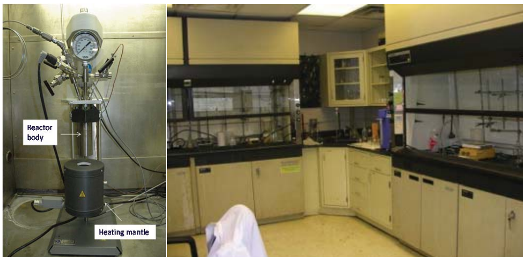
Figure 6.—(left) 100 mL stirred batch reactor, maximum temperature 500 °C, maximum pressure 5000 psi; (right) catalyst processing laboratory—facility for running CWAO reactor.
