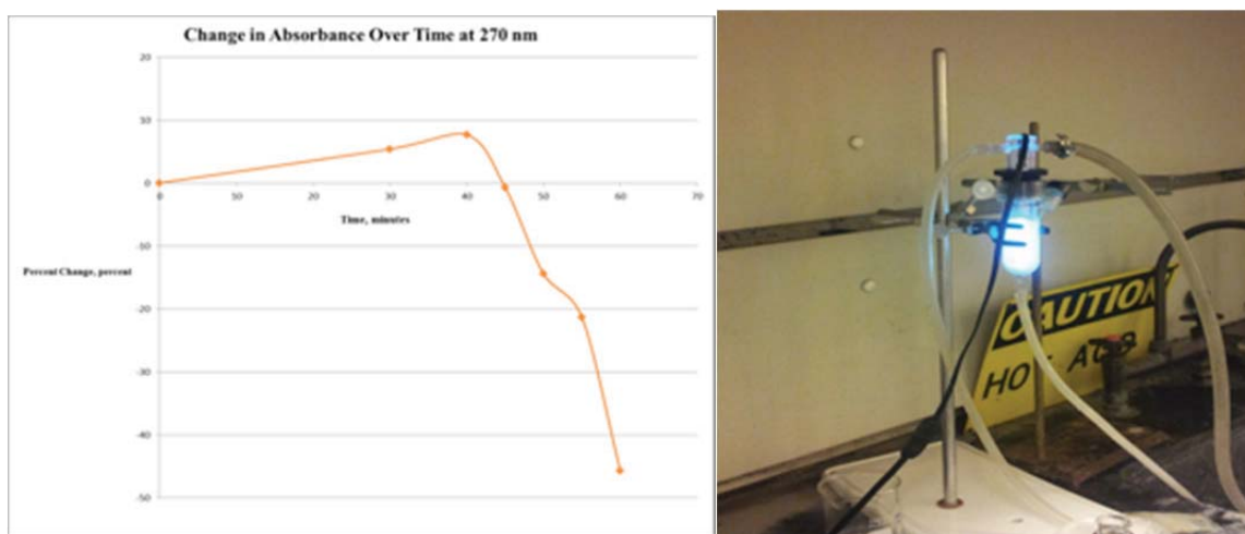
Figure 7.—Photocatalysis of phenol—(left) UV-Vis plot showing photodecomposition; (right) reactor.
