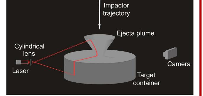
A capability afforded by the vertical gun is the measurement of ejection velocities from craters formed in granular, strengthless targets, like sand.
