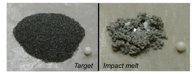
The LGG is capable of duplicating impact conditions in the asteroid belt. As an example, this powdered gabbro (a dark, igneous rock often polished and used for kitchen counters) was impacted with a ceramic sphere (shown for scale) at 5.5 km/s, fast enough to melt a large fraction of the rock. Such impact melts could be important components of asteroid soils.
