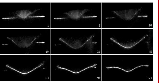
Glass spheres 50  $\mu$ m across (about as wide as a human hair) made these tracks in a three-layer aerogel target when they impacted at 6 km/s. Remnants of one of the particles can be seen at the end of the track in the center of the right edge. Experiments like this were performed during development and testing of the Stardust aerogel, which ultimately captured cometary dust.
