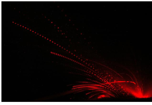
An example of a picture taken during the impact of a 3.2 mm (1/8'') glass sphere into a coarse sand at 2.45 km/s.
