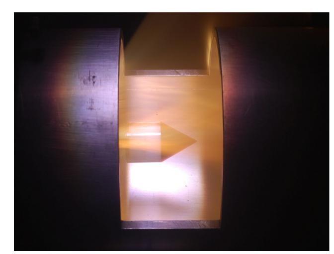
The projectile must impact the target with its front parallel, or nearly so, to the face of the target. This is determined by photographing the projectile in flight and measuring its tilt in two photographs, taken 90° from each other.
