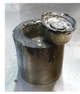
A stainless-steel target assembly after impact. The sample is still contained in the smaller sample assembly; it will be mounted in a lathe, excess metal will be machined away, and the sample recovered for a variety of possible analyses.
