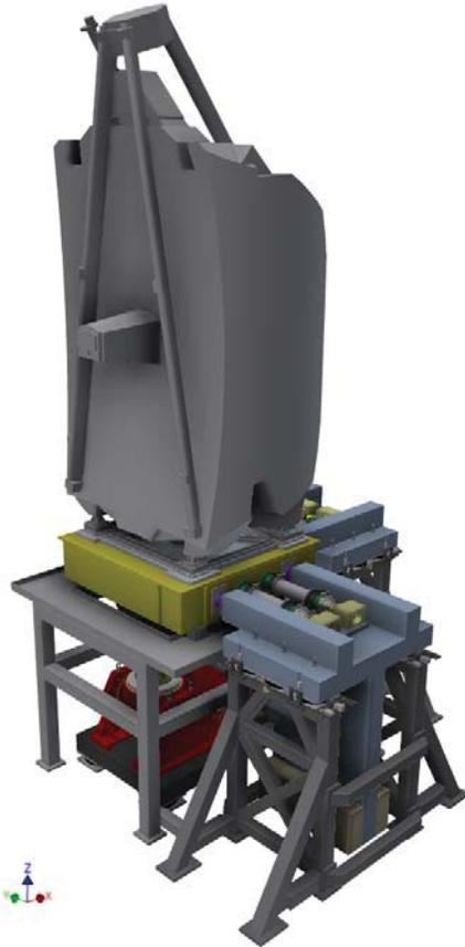
*Figure 6: Vertical System with OTIS Payload Attached*
