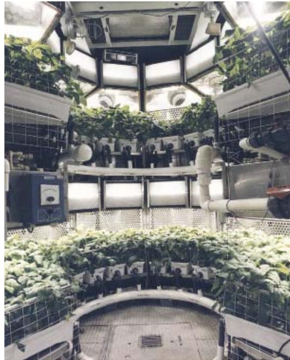
Fig. 1. NASA's Biomass Production Chamber at Kennedy Space Center with soybean crop. Two of the four shelves are shown; the chamber provided 20 m<sup>2</sup> of growing area in a closed atmosphere
