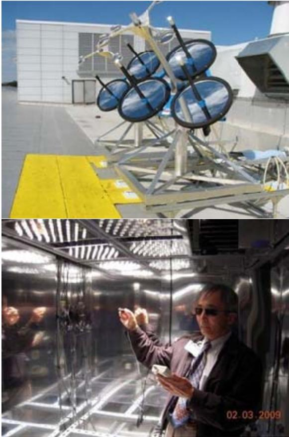
Fig. 6. Top: Solar concentrators on the roof of the Space Life Science Laboratory at Kennedy Space Center, Florida; Bottom: Takashi Nakamura, Physical Sciences Inc., making measurements of light delivered from the concentrators (Nakamura et al., 2009).
