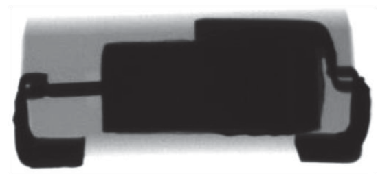
Typical X-ray view showing location of internal part of cathode terminal
