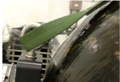
Figure 2 - RTA lifting eyelet with nylon loop of the RTA strap.
