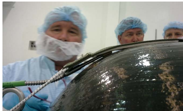
Figure 4 - The thermocouple secured to the RTA under the strap. Non-slip material provides tension and prevents the thermocouple from sliding off the tank surface.
