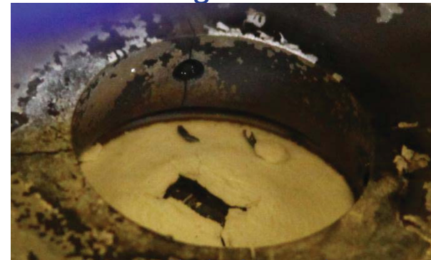
Coating spalled after 40 hr test
