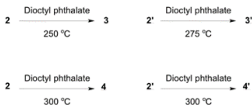
Figure 3. Reaction scheme for the conversion of the single-source precursors to \text{CuInS}_2 or \text{CuInSe}_2 .
