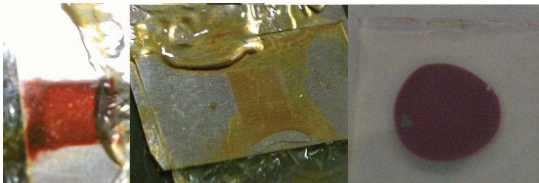
Figure 11. Left to right: Dysol Paste; Old pH = 2 aqueous ink with 15 nm \text{TiO}_2 ; new aqueous ink.
