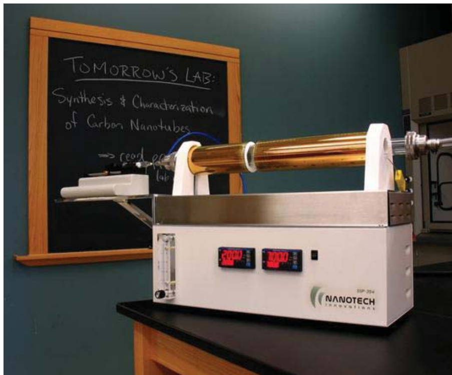
Figure 22. Nanotech Innovations LLC's commercially available MWNT production reactor - SSP-354.
