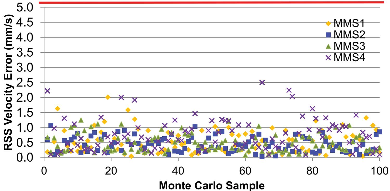
Definitive velocity error one orbit after first maneuver well under 5 mm/s velocity error threshold
