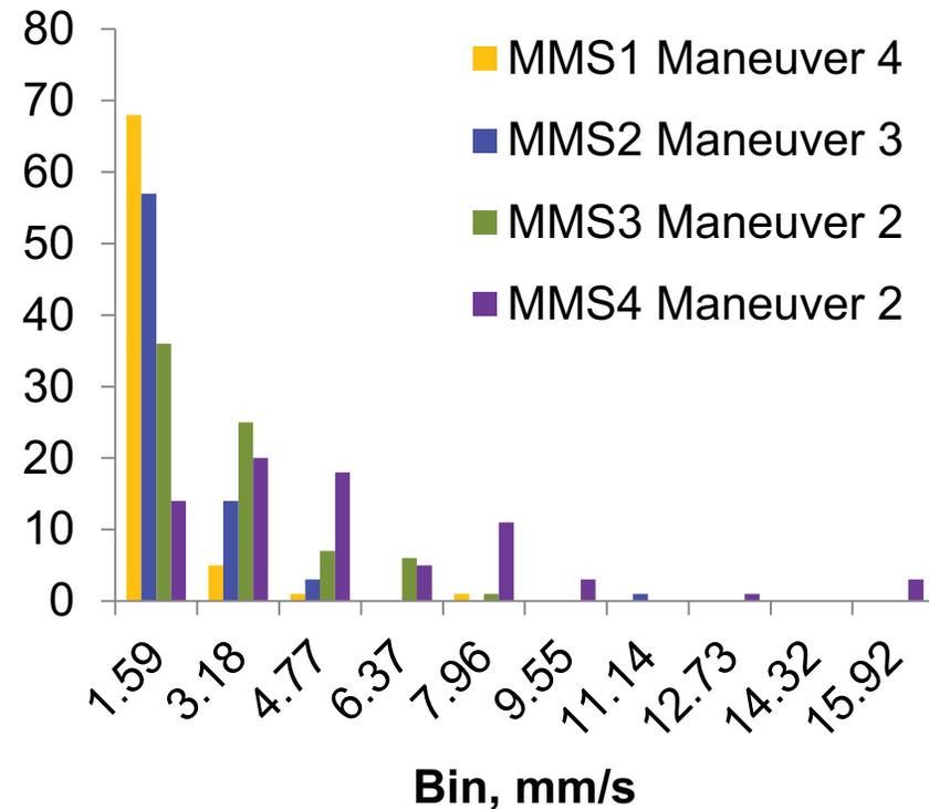
First maneuver and MMS3 and MMS4's second maneuver have consistent and significant errors greater than 5 mm/s
