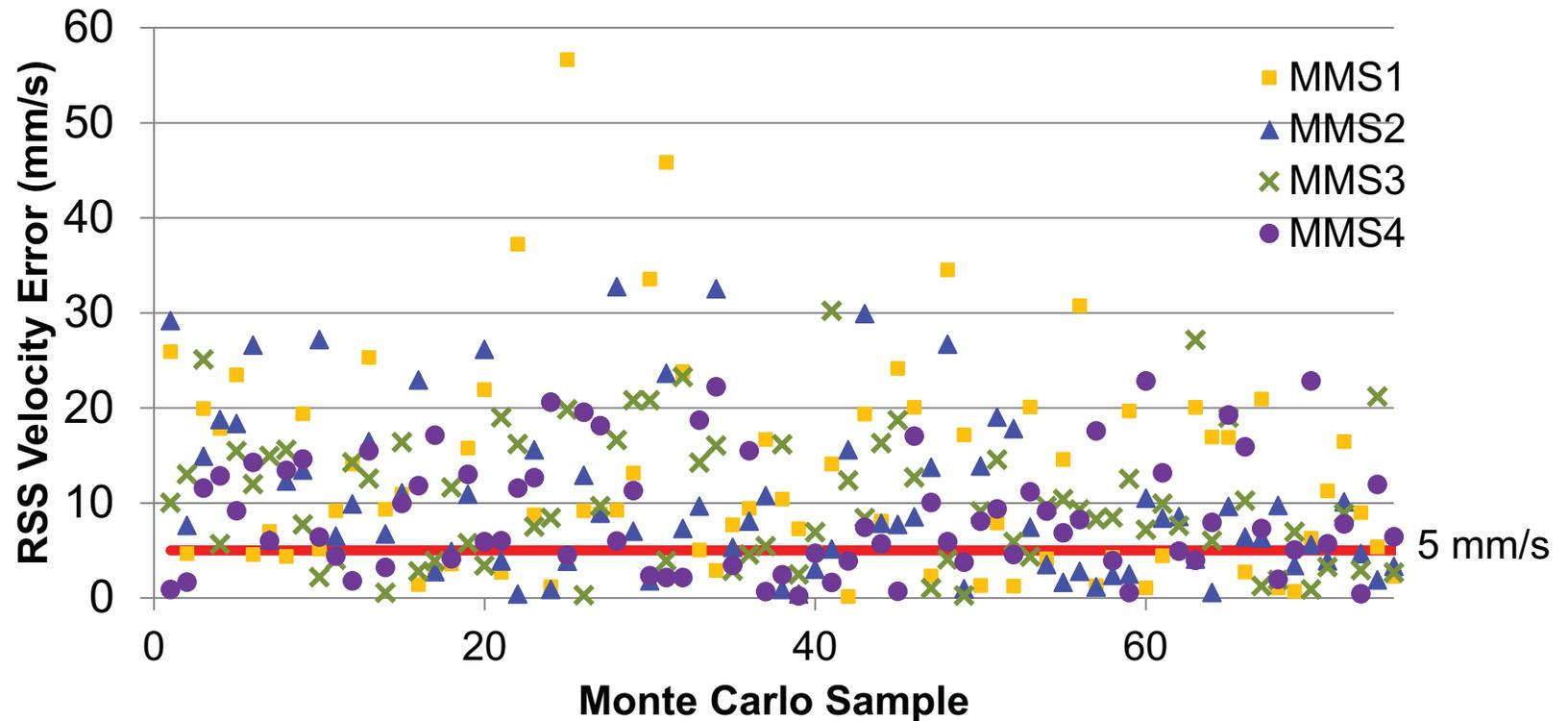
Predictive velocity error one orbit prior to 1<sup>st</sup> maneuver well over 5 mm/s velocity error threshold, but under 1% of maneuver magnitude
