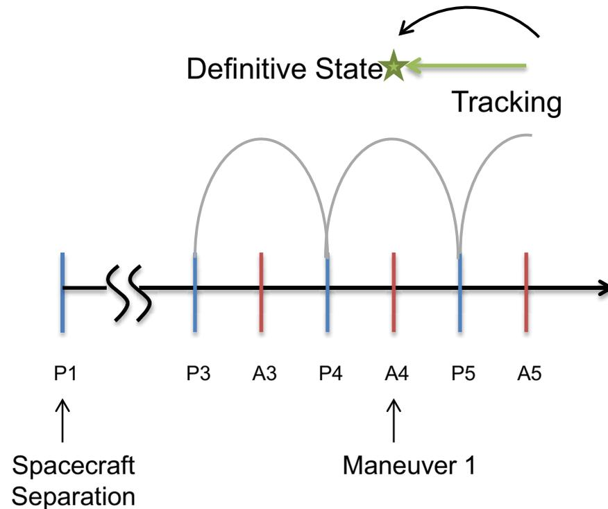
An accurate post-maneuver state is needed within 1 orbit to calibrate thruster performance and plan for the upcoming maneuvers
