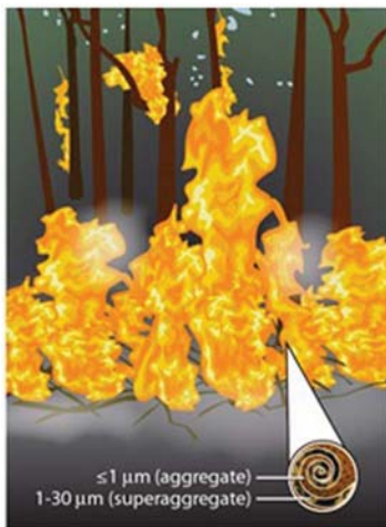
Figure 6 | Schematic (drawn using Adobe Photoshop™) hypothesizing the soot superaggregate formation mechanism in wildfires. Particle residence times are enhanced for cluster-dilute aggregates that get trapped into one of the many vortices inside a large-scale, turbulent flame. This facilitates increase in particle volume fractions and percolation of aggregates into superaggregates inside the flame.
