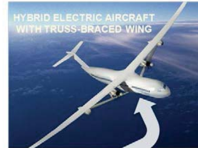
Gas turbine-battery hybrid
