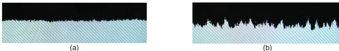
Figure 9.—Monte Carlo predicted Kapton H erosion profiles for a: (a) 300 °K thermal energy plasma and (b) 0.26 eV hyperthermal plasma.
