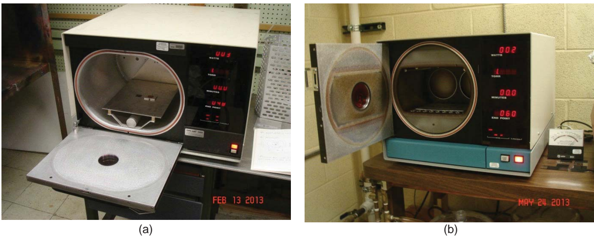
Figure 2.—LF plasma ashers: (a) LF-6, 30 kHz and (b) LF-5, 35 kHz.
