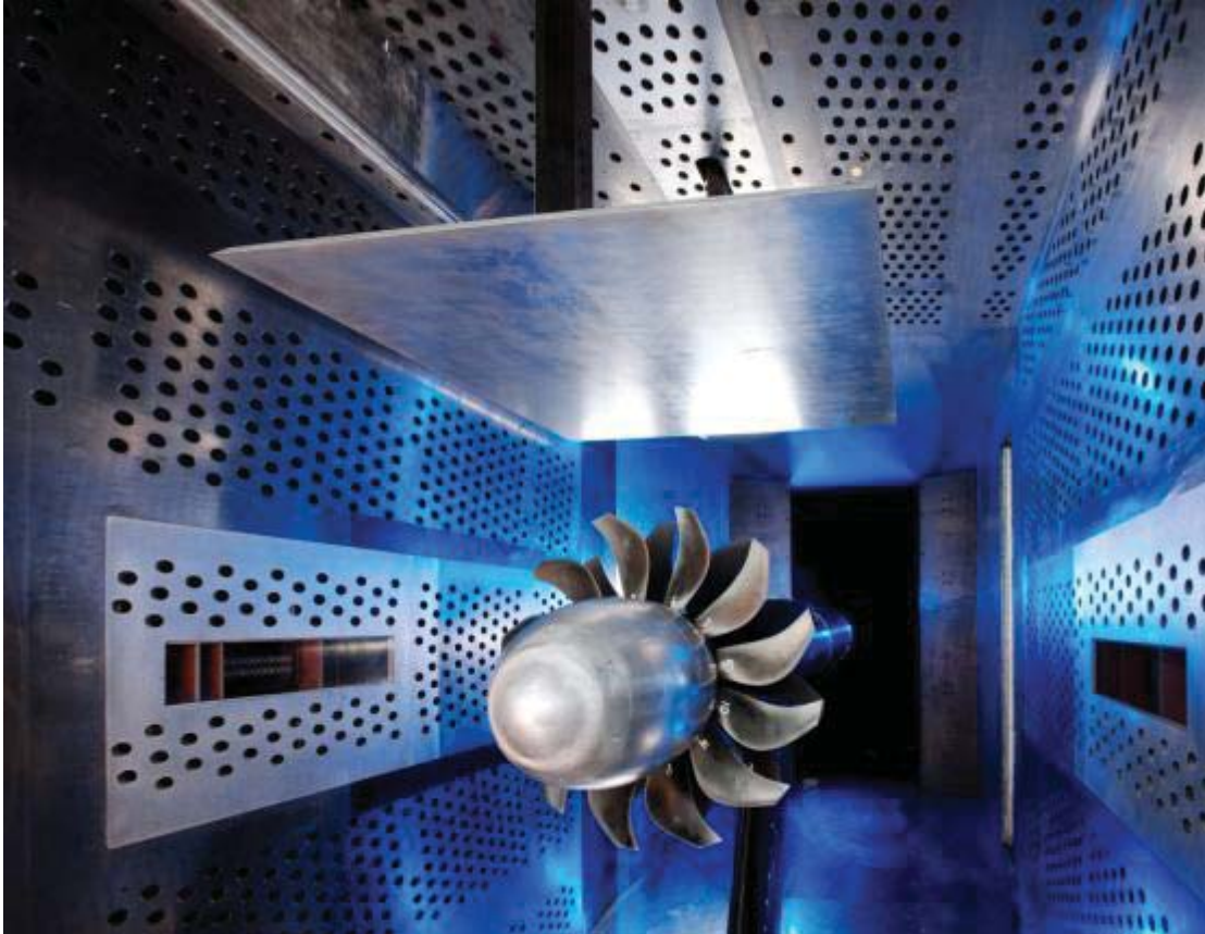
Figure 3.—ORPR installed in 8- by 6-ft SWT with Kulite plate above.
