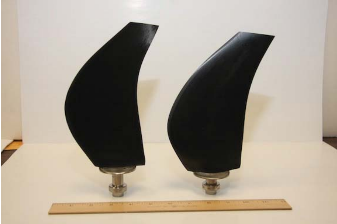
Figure 1.—F31/A31 rotor blades, shown with a 1 ft ruler for scale.
