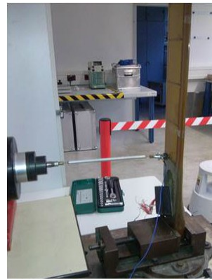
Figure 2. Blade frequency measurement setup at DLR laboratory.
