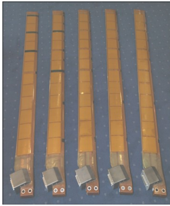
Figure 1. STAR Blades manufactured at DLR Braunschweig laboratory
