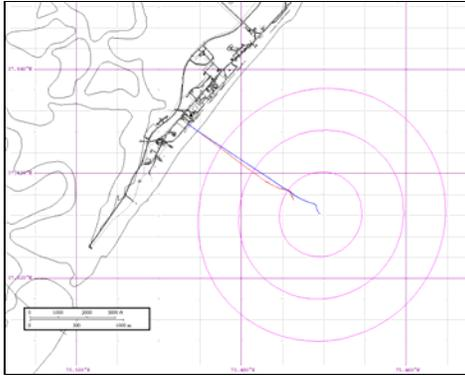
Figure 16. Comparison of Pre-Flight Predicted Ground Track with Flight Data. Circles Indicate Pre-Flight Standard Deviations of Dispersed Monte Carlo Simulations.
