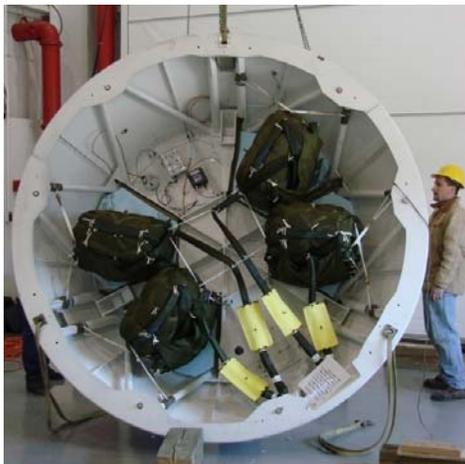
Figure 9. MLAS Crew Module Recovery Parachutes in Forward-Bay Cover
