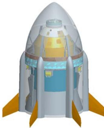
Figure 5. Final Side-Mounted Escape Motor MLAS Concept with Aerodynamic Fins for Coasting Flight Stability
