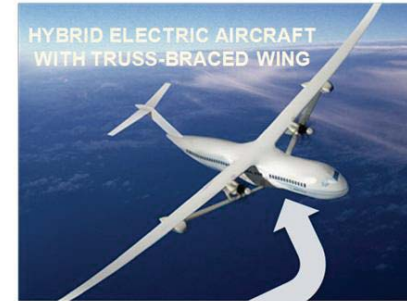
Gas turbine-battery hybrid
