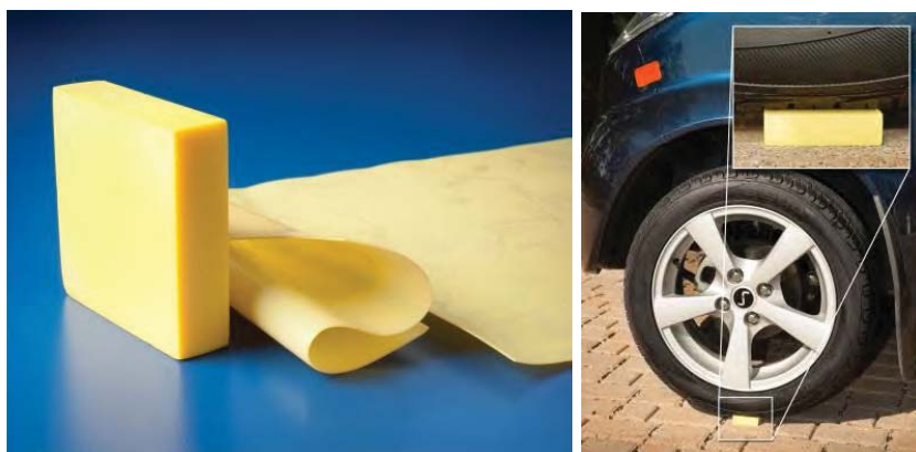
Figure 23. Polyimide aerogels cross-linked with TAB shown fabricated as flexible thin films or molded to a net shape. (Reprinted with permission from Publication 7. Copyrights 2012 American Chemical Society).
