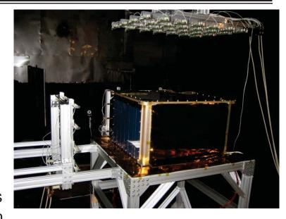
By using the Structural Test Article (STA) to define this test setup in advance, the project reduced the time needed for thermal vacuum cycling and performance verification of the Flight payload.
