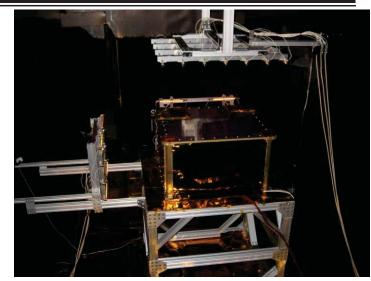
The heat flux values that the lamps are required to produce was calculated from the SCaN Testbed detailed Thermal Desktop model.
