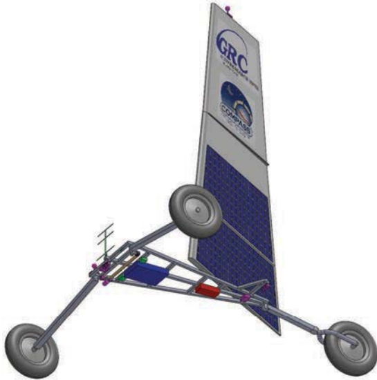
Fig. 2: Perspective view of the Zephyr Venus Rover as deployed on the surface (underside view)
