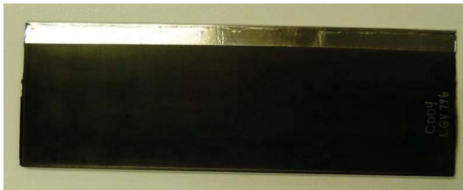
Figure 10: Prepared leading edge test article
