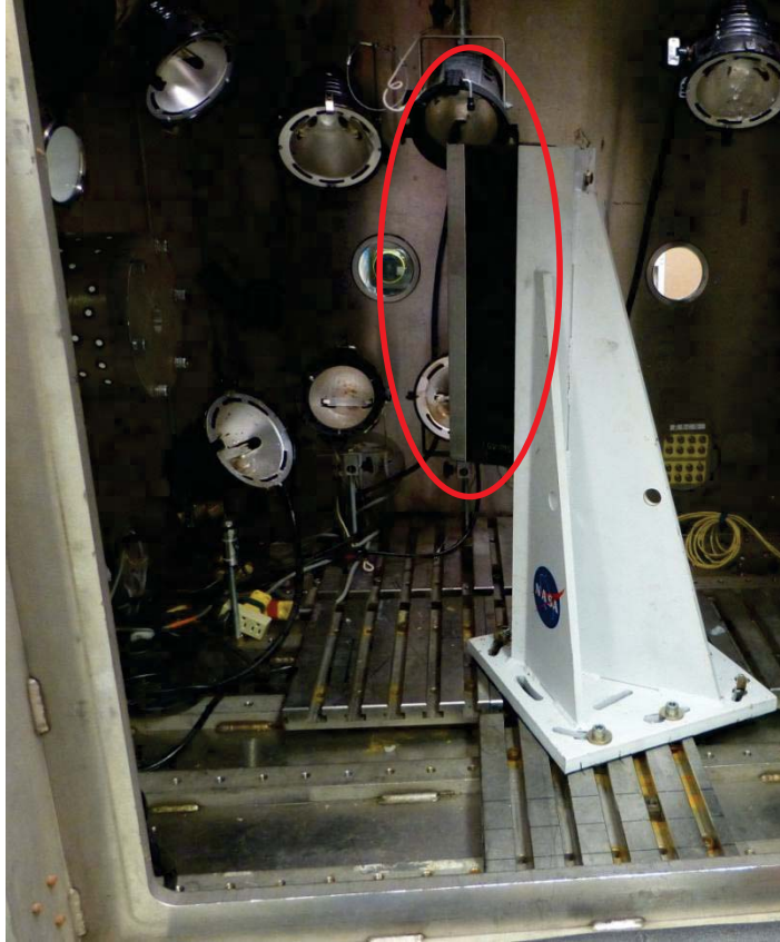
Figure 11. Impact testing fixture secured in impact chamber
