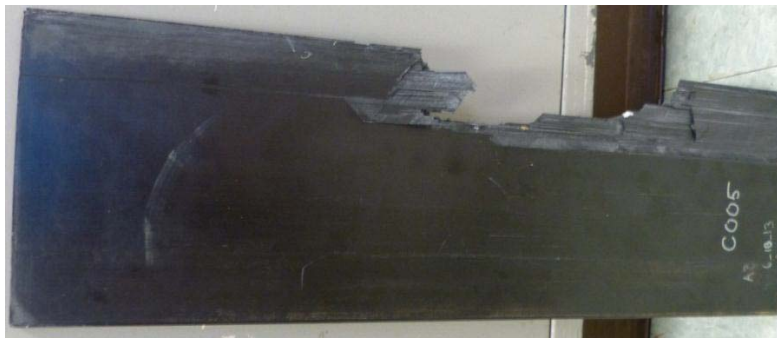
Figure 14. C005 Impact Damage
