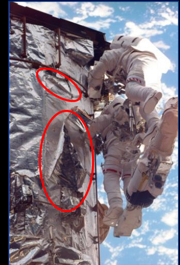
Radiation induced embrittlement & cracking of Teflon insulation (6.8 yrs)
