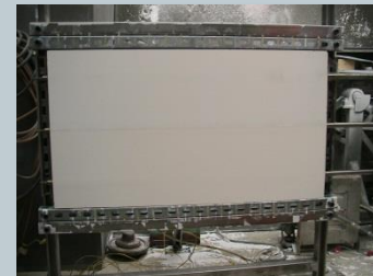
PS-16 thermal control coating on test radiator
