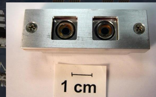
Post-flight photo of ram ITO Experiment
