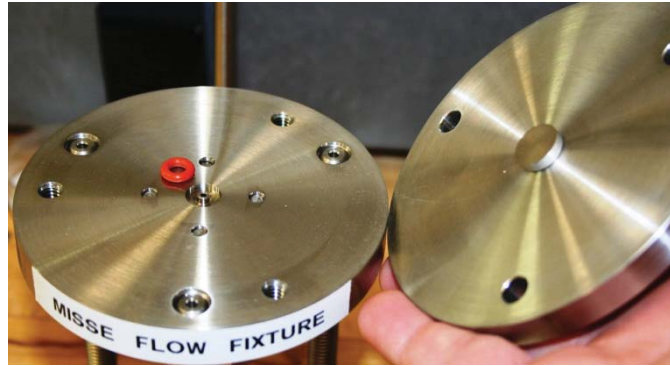
Figure 4.—Plates of the MFF, a #2-106 O-ring, and anodized aluminum alloy counter-face at the center of the top plate.
