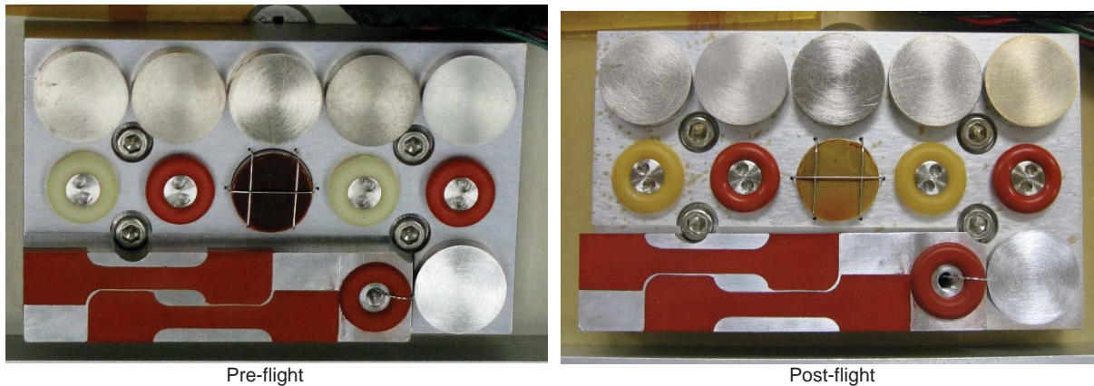
Figure 2.—Pre and post-flight images of the 4 cm wide, windward MISSE-7 Seals Experiment assemblies.
