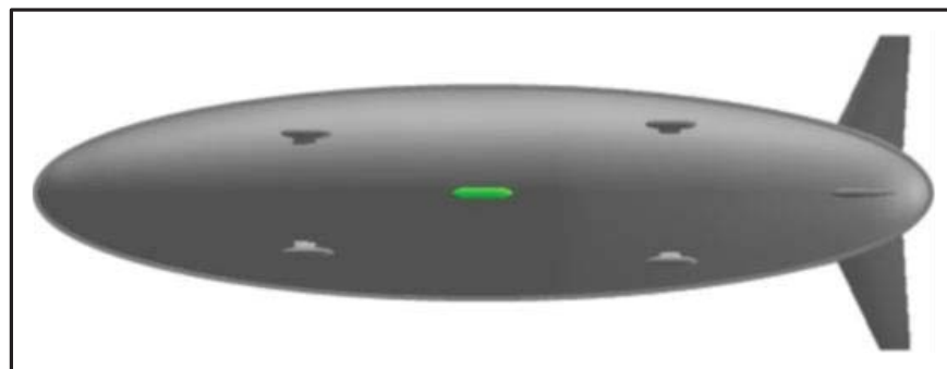
Figure 20. LTA-1080 bottom view schematic: propulsion and payload (green) pods.
