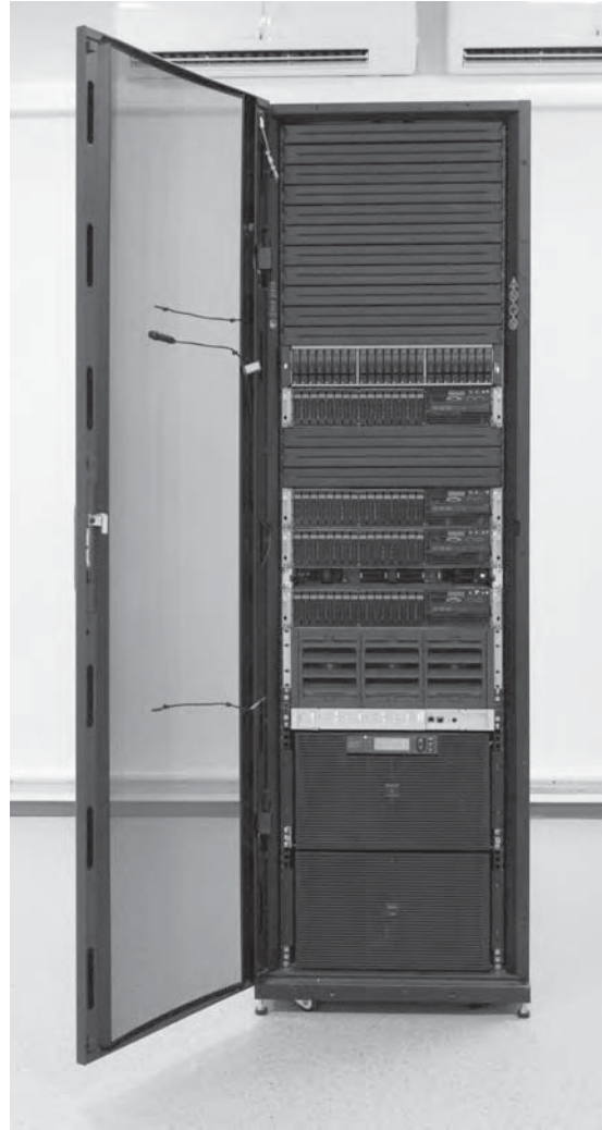
Fig. 2 View of the high-performance computing cluster based on the hybrid blade servers.
