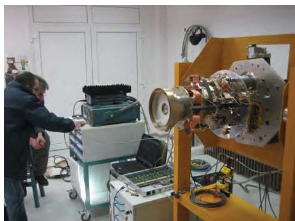
Fig. 5 Tri-band (S/X/Ka) receiver, designed and built at the laboratories in Yebes Observatory.
