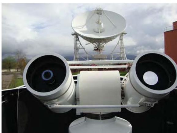
Fig. 3 “Sazhen-TM” SLR system at Zelenchukskaya observatory observed 744 passes of Lageos, GLONASS et al. and obtained 1278 normal dots.
