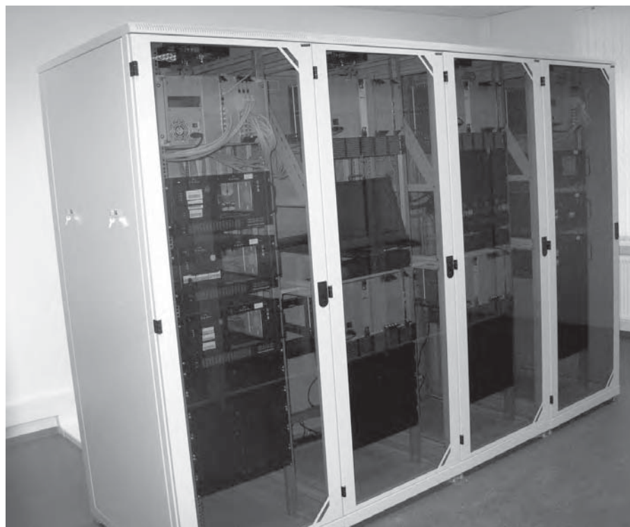
Fig. 1 View of the six-station ARC correlator, showing four racks containing (left to right) signal distribution and synchronization system (SDSS) and three Mark 5B playback units, two correlator crates and KVM, three correlator crates, and one more cabinet with SDSS and three Mark 5B playback units.
