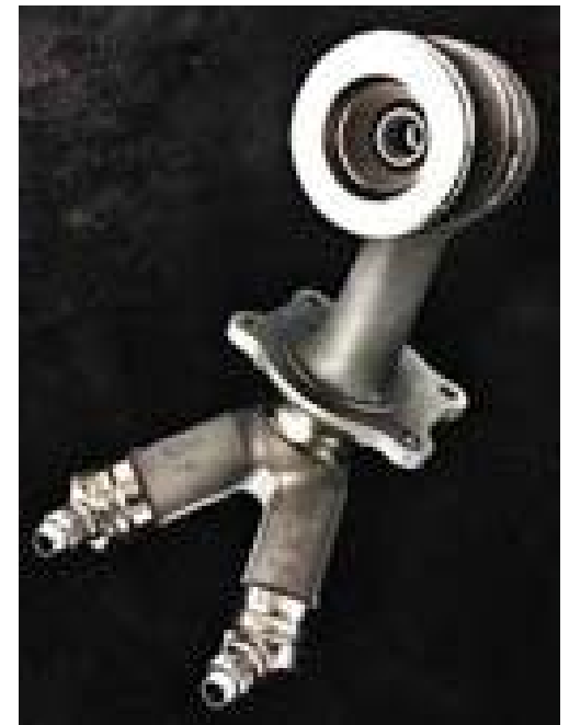
GE Leap Engine fuel nozzle. CoCr material fabricated by direct metal laser melting (DMLM), GE's acronym for DMLS, SLM, etc.
