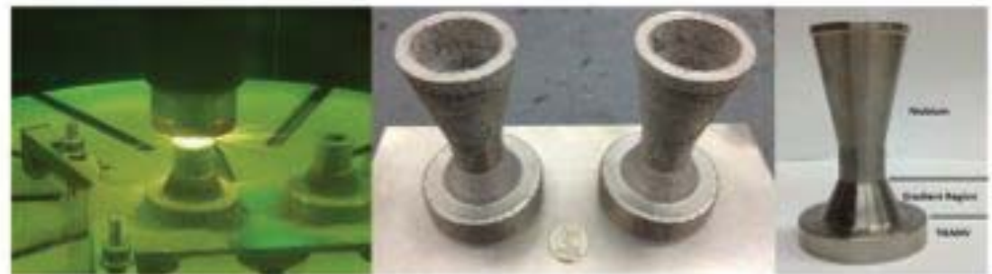
Prototype titanium to niobium gradient rocket nozzle
