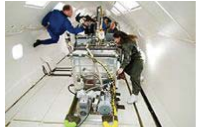
EBF3 system during parabolic flight testing
