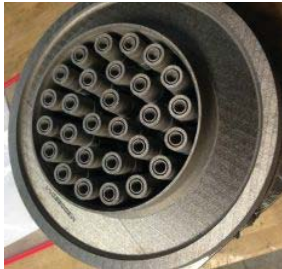
28 element Inconel 625 fuel injector built using SLM process
