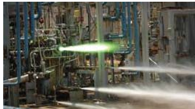
28 element Inconel 625 fuel injector built using SLM process
