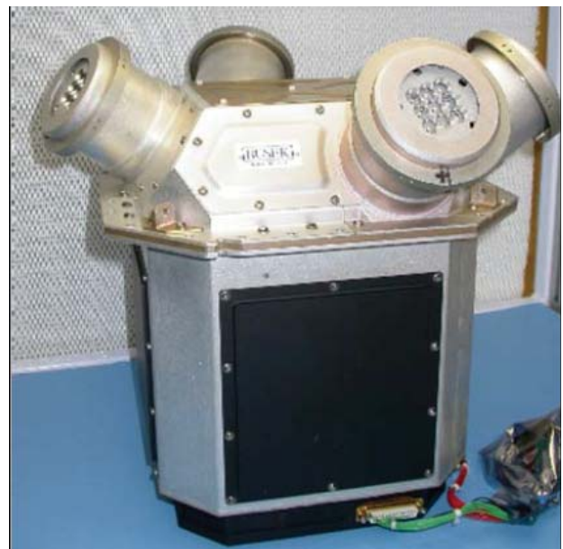
Figure 3: Electrospray thrusters for the Laser Interferometer Space Antenna (LISA) Pathfinder
