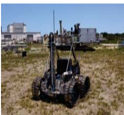
Figure 2. RESOLVE Payload and Resource Prospector Rover Field Test Unit. The LAVA subsystem is depicted in the black box on the rover. Photo credit: NASA/Dmitri Gerondidakis
