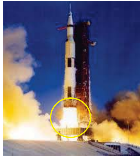
The 5 F-1 Liquid Rocket Engines on the Saturn V Moon Rocket had a combined thrust of over 7.5 Million Pounds at Lift-off
