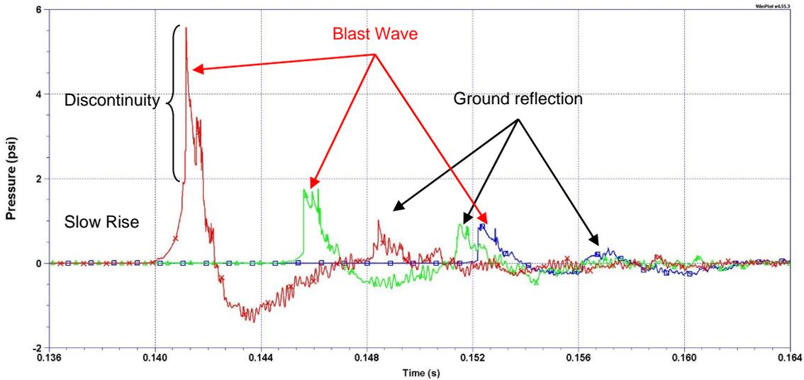
**Figure 8: HUCTA 101, Bag at 65.4% H<sub>2</sub> by Volume with O<sub>2</sub>**
