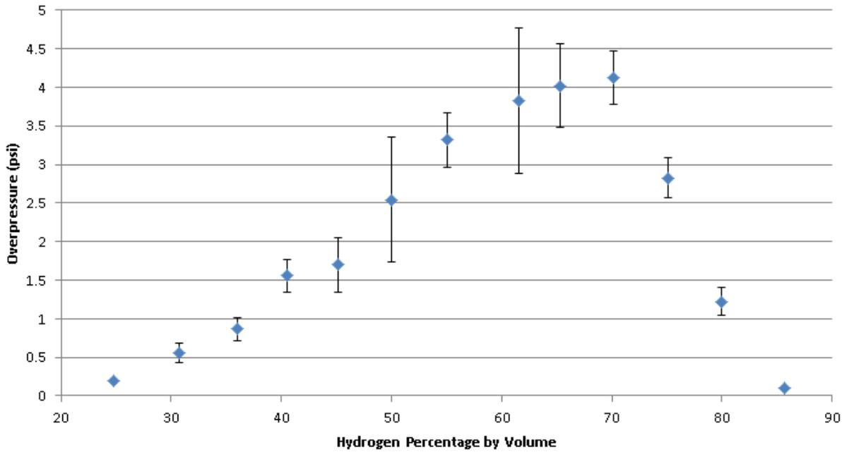
**Figure 17: Average Overpressure vs. Concentration for small bags of H<sub>2</sub>/O<sub>2</sub> at 42'' from the Center of Explosion**
