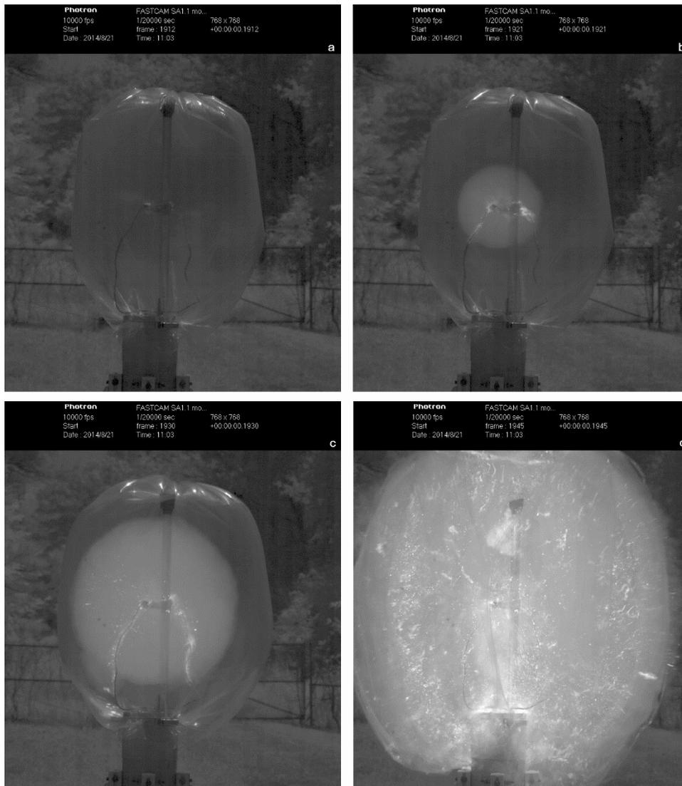
**Figure 4: Typical results of high speed video for small bag combustion at 67.5% hydrogen by volume (a) t = 0, (b) t = 9ms, (c) t = 18 ms, (d) t = 33 ms after ignition by spark.**
