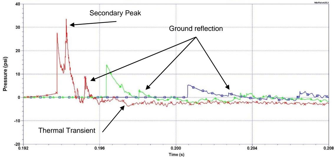
**Figure 10: HUCTA 177, Balloon at 67% H<sub>2</sub> by Volume with O<sub>2</sub>**
