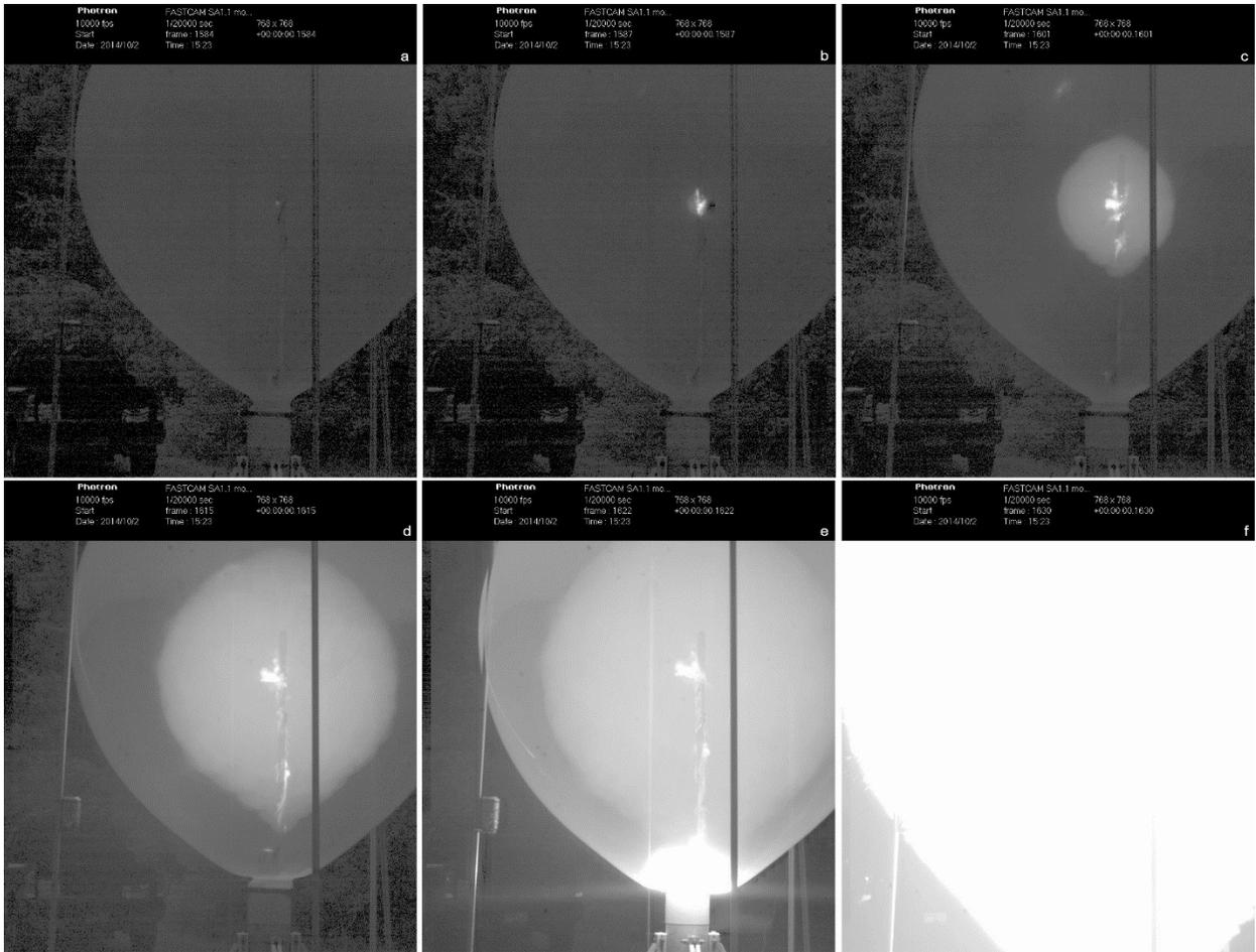
**Figure 5: Typical results of high speed video for balloon combustion at 64% hydrogen by volume (a)  $t = 0$ , (b)  $t = 3$ ms, (c)  $t = 17$  ms, (d)  $t = 31$  ms, (e)  $t = 38$  ms, (f)  $t = 46$  ms after ignition by spark.**
