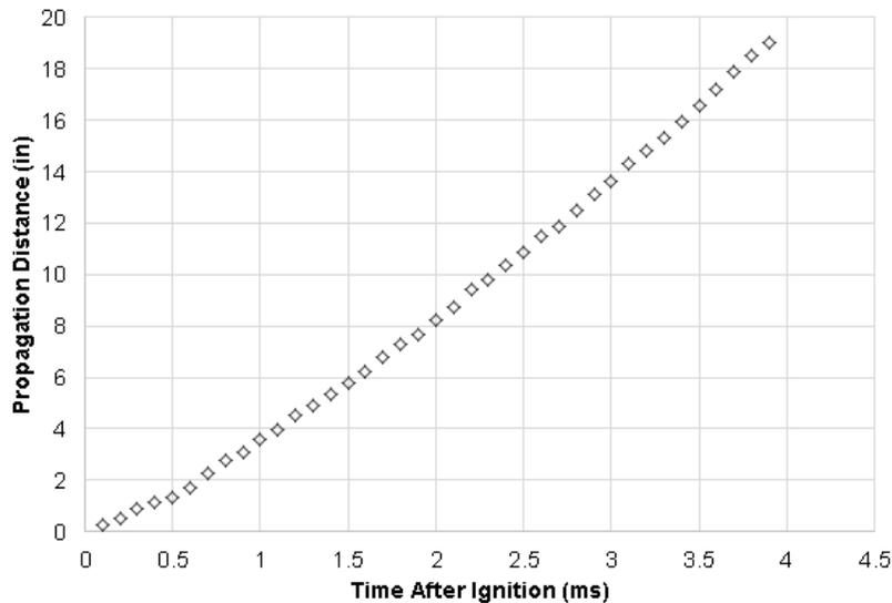
**Figure 7: Large Balloon Flame Propagation vs. Time for Stoichiometric H<sub>2</sub>/O<sub>2</sub>**
