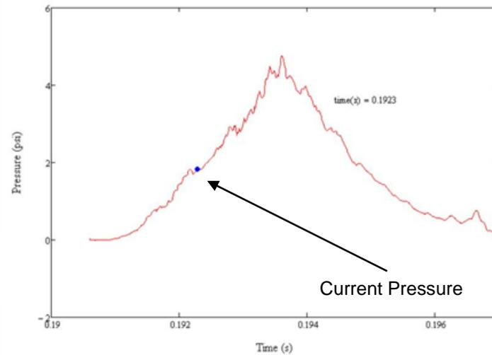
Figure 13: HUCTA , Bag at 68.6% H<sub>2</sub> by Volume with O<sub>2</sub> and Internal Sensor, t = .1923s
