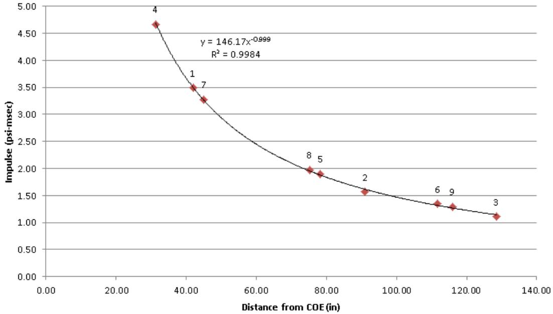
**Figure 16: HUCTA 50, Bag at 60.8% H<sub>2</sub> by volume with O<sub>2</sub>, Impulse vs. Radial Distance from COE**
