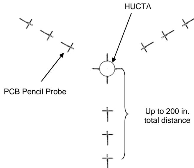
**Figure 3: HUCTA with Sensor Configuration**
