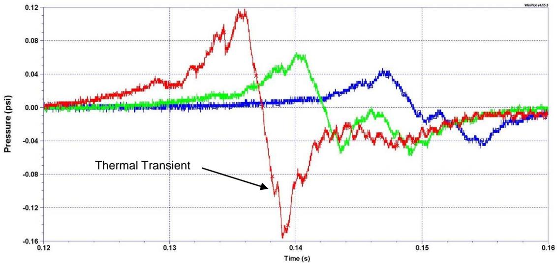
**Figure 9: HUCTA 125, Bag at 30.1% H<sub>2</sub> by Volume with Air**
