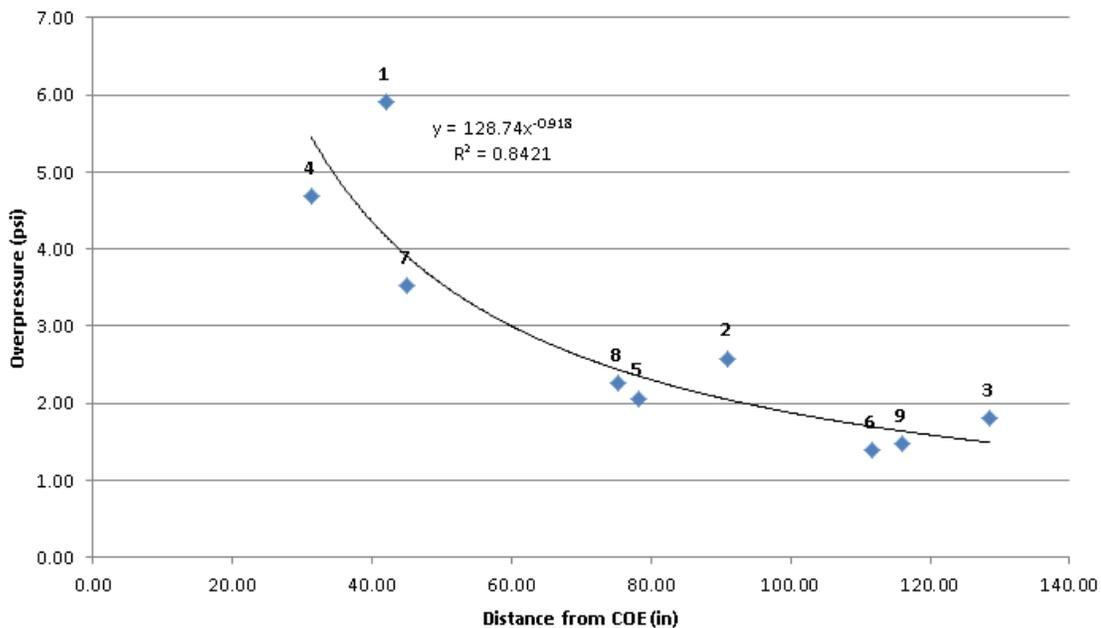
**Figure 15: HUCTA 50, Bag at 60.8% H<sub>2</sub> by volume with O<sub>2</sub>, Peak Overpressure vs. Radial Distance from COE**
