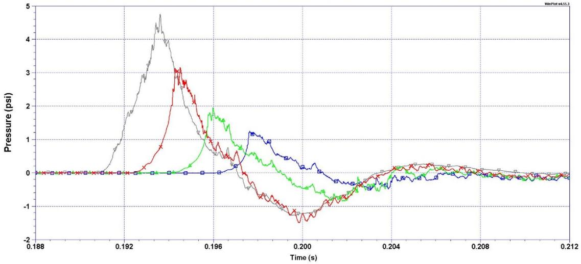
Figure 11: HUCTA 133, Bag at 68.6% H<sub>2</sub> by Volume with O<sub>2</sub> and Internal Sensor
