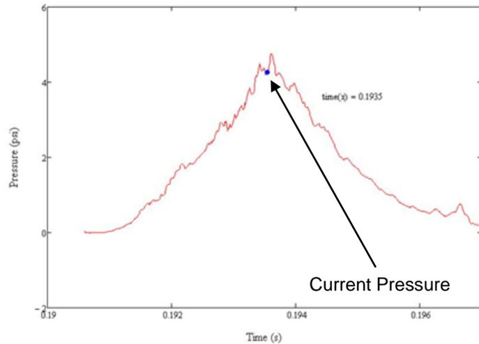
**Figure 14: HUCTA 133, Bag at 68.6% H<sub>2</sub> by Volume with O<sub>2</sub> and Internal Sensor, t = 0.1935s**
