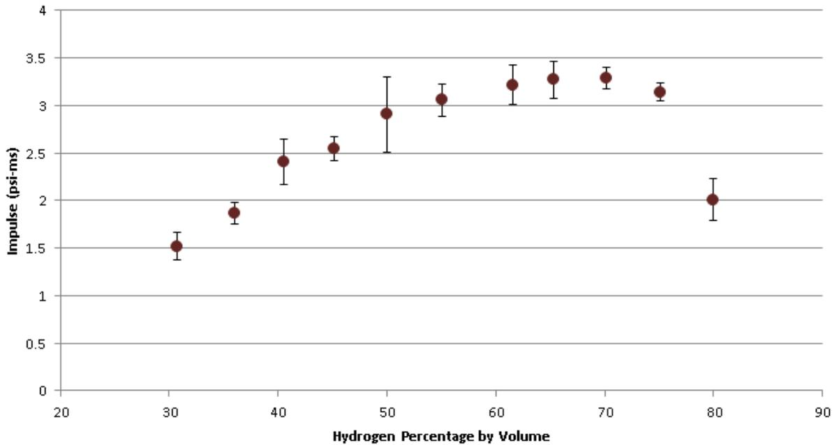
**Figure 18: Average Impulse vs. Concentration for small bags of H<sub>2</sub>/O<sub>2</sub> at 42'' from the Center of Explosion**
