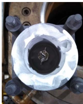
Above left/right: 7 channel W-VO 2 FE during HIP process
