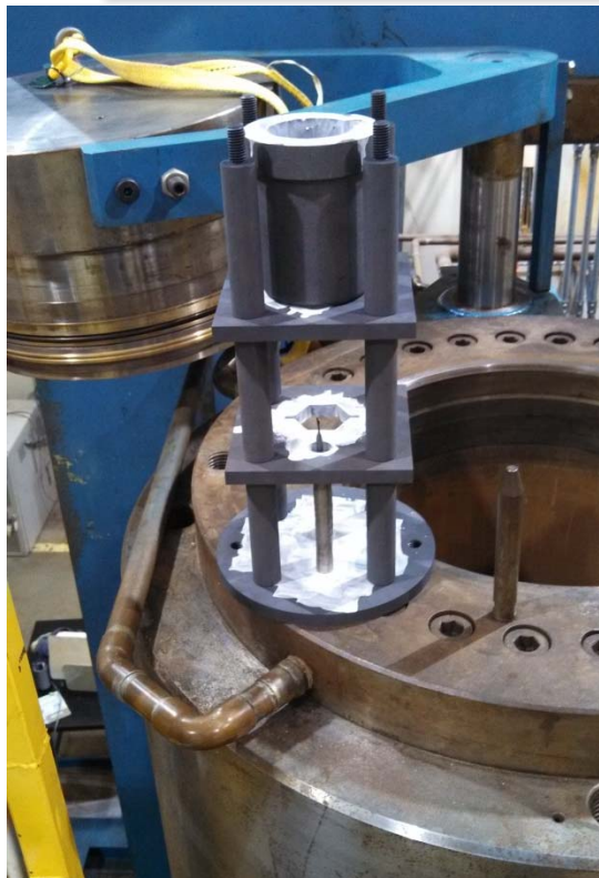
Above left/right: 7 channel W-VO 2 FE during HIP process
