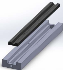
Right: Layoff base / Graphite insert
