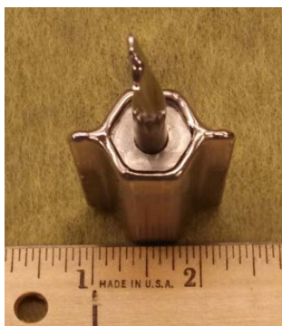
Above left/right: 7 channel W-VO 2 FE during HIP process
