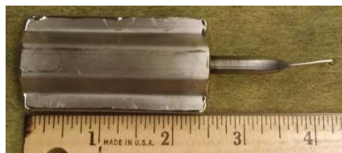
Left & above: LANL sample post fill and closeout prior to shipping
