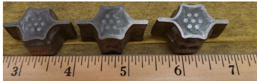
Above/Below: 7 channel WVO 2 fuel element post HIP and cross sections
