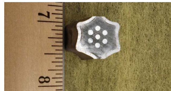
Above/Below: 7 channel WVO 2 fuel element post HIP and cross sections
