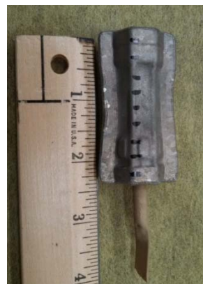
Above/Below: 7 channel WVO 2 fuel element post HIP and cross sections
