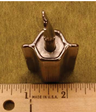
Above left/right: 7 channel W-UO 2 FE during HIP process
