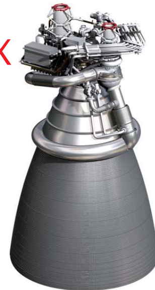
J-2X Rocket Engine for Constellation
