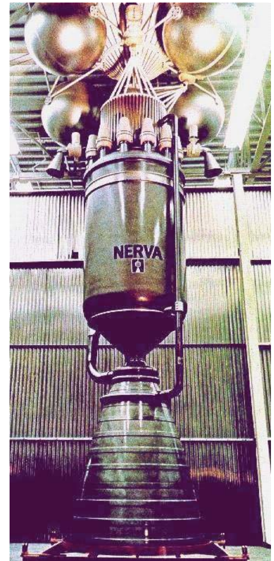
NERVA Nuclear Thermal Rocket Prototype
