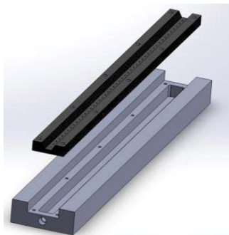
Right: Layoff base / Graphite insert
