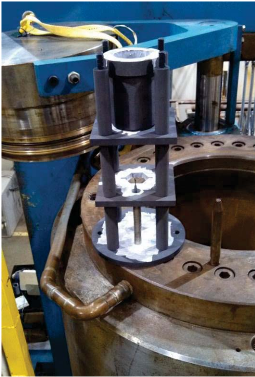
Above left/right: 7 channel W-UO 2 FE during HIP process
