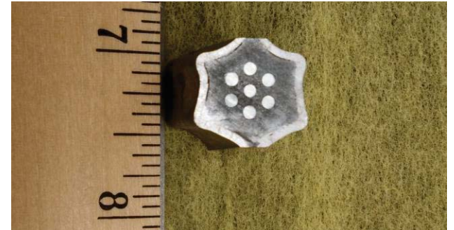
Above/Below: 7 channel WUO 2 fuel element post HIP and cross sections
