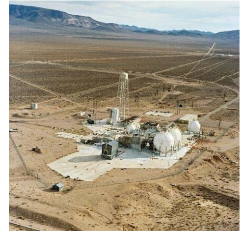
Test Cell "C" With two 500,000 gallon dewars of LH2
