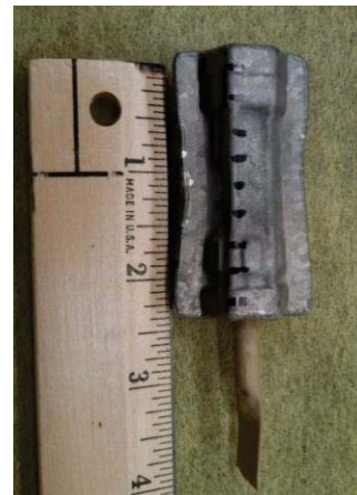
Above/Below: 7 channel WUO 2 fuel element post HIP and cross sections
