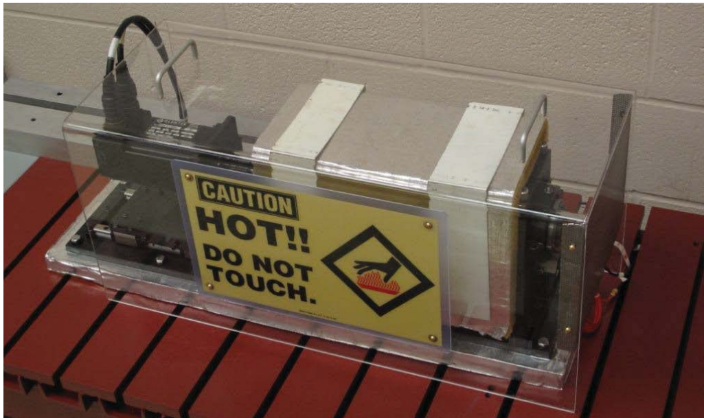
Figure 1 – Grease Degradation Rig Setup with Insulation and Guard Shield Installed
