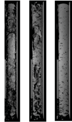
Sight Glass during Line Chilldown
