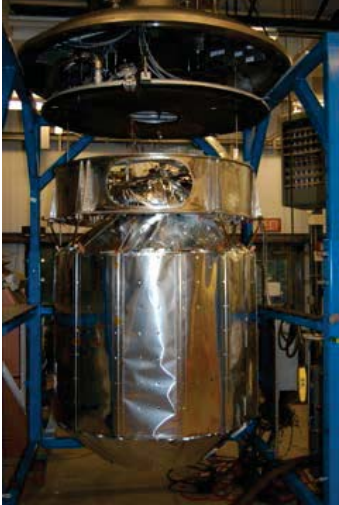
LH2 Active Cooling – Thermal Test (RBO) and Acoustic Test (VATA)
