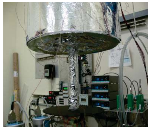
(MLI) Penetration Heat Leak Study
