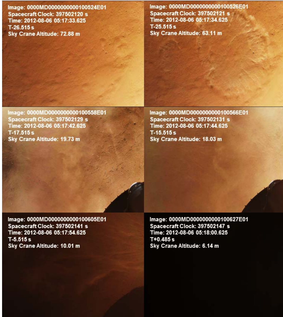
Figure 2: MARDI images taken during descent phase. Correlated MARDI images with trajectory data shows rocket thruster – soil interaction occurs at roughly 63 meters above the surface at 25 seconds before touchdown. Significant erosion occurs within the last 15 seconds.
