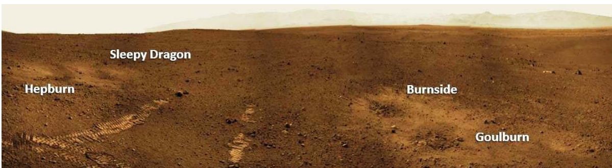
Figure 6: Landing Site Panoramic. Two pairs of craters formed by the Sky Crane maneuver are visible in this composite panoramic.
