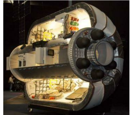
One example of an inflatable habitat, the proposed Bigelow Aerospace BA-330. Image credit: AP
