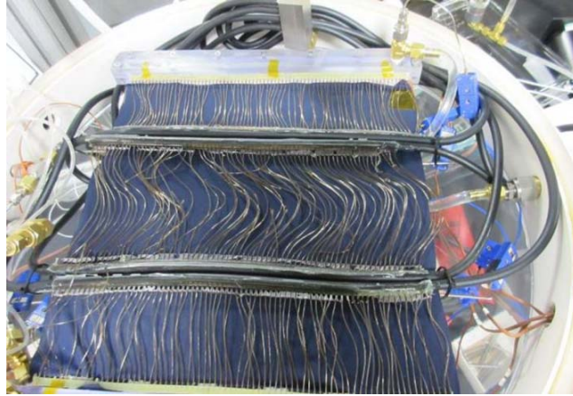
(b) Latent Cooling Tubes
