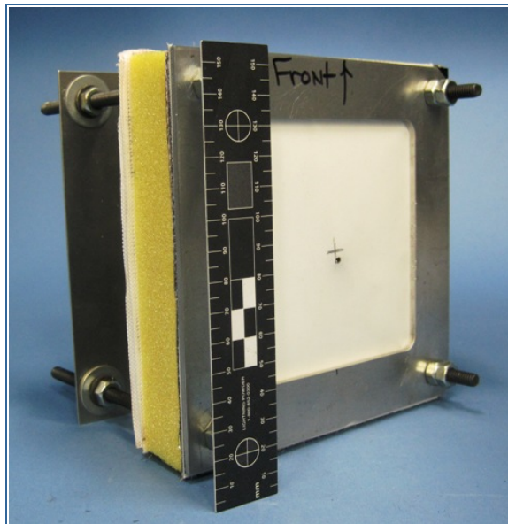
Figure 2.– Hypervelocity impact tests were performed to demonstrate the effectiveness of the toughened thermal blankets.
